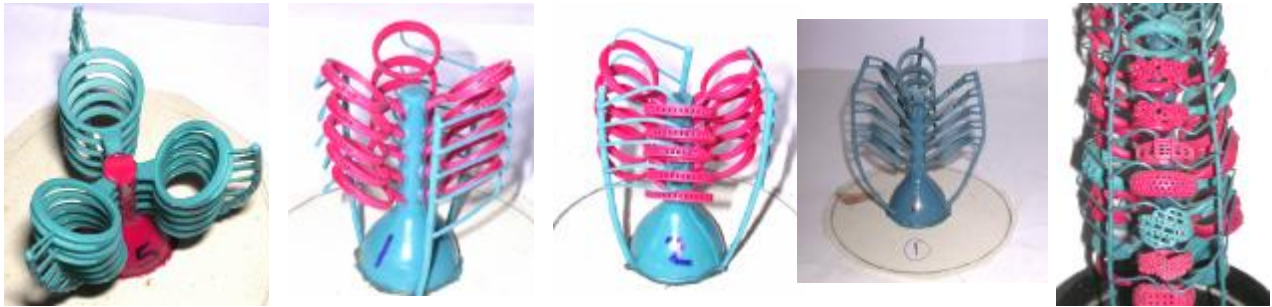
Fig. 6:- Misc. EXAMPLES OF CONNECTING THE GATES
