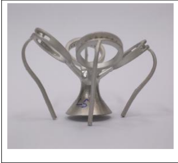
Fig. 14 SUCCESSFUL CASTING OF TEST TREE
