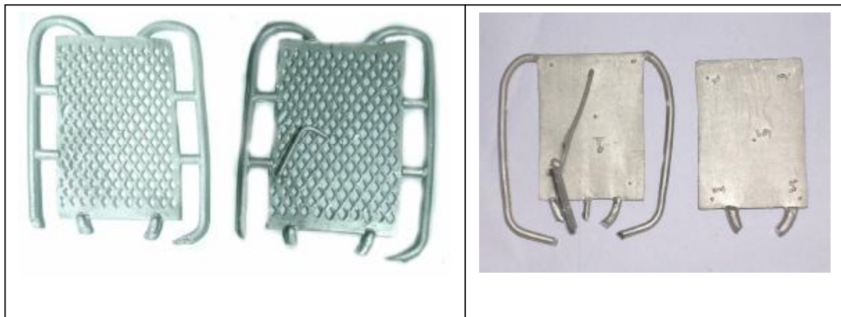
Fig. 13. GRID STRUCTURE AND THIN WAFER CASTED IN PLATINUM
