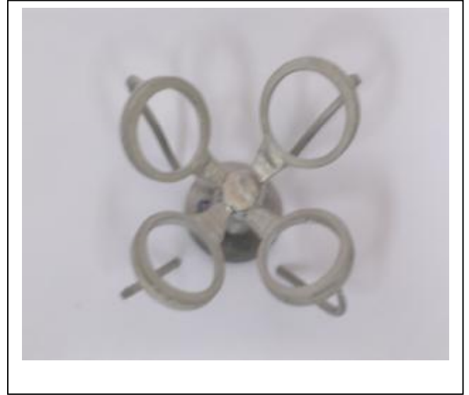
Fig. 14 SUCCESSFUL CASTING OF TEST TREE
