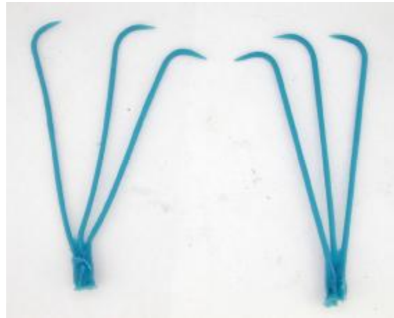
Fig. 11(B):- CONNECTING GATES KEPT READY FOR ATTACHMENTS.
