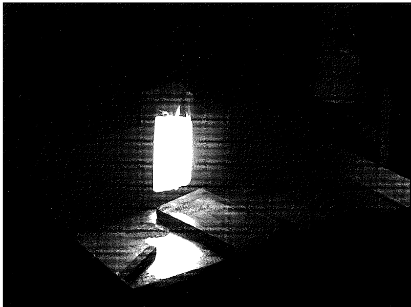
Figure 6: A hot solidified platinum alloy ingot.
