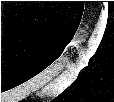
Figure 24: SEM of weld joint of Pt-Co-Cu ring
