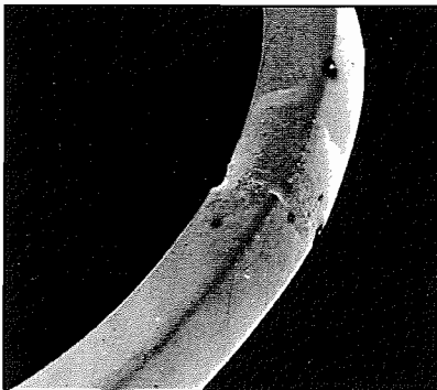
Figure 23: SEM of weld joint of Pt-Ru ring
