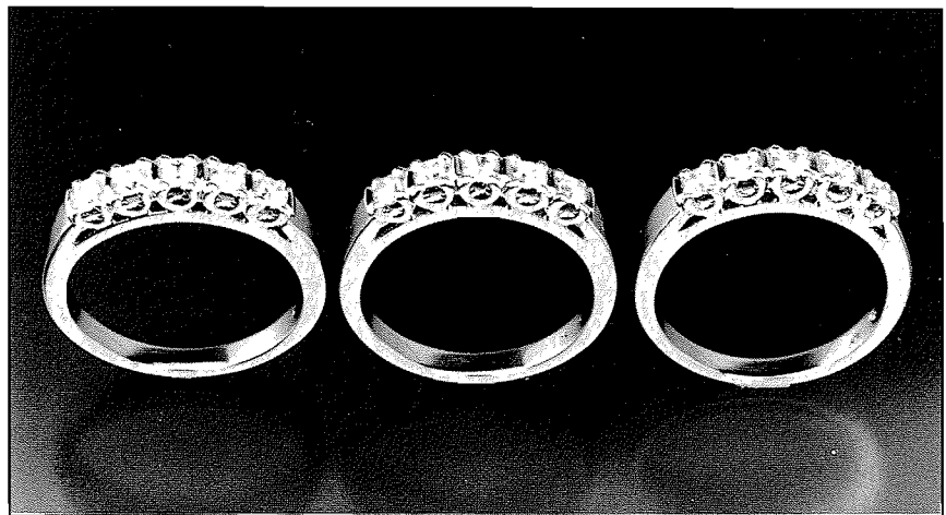
Fig. 25: (Left to right) Finished "fishtail" ring mountings in Pt-Co, Pt-Ru, and Pt-Ir alloys
