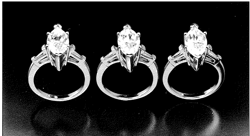
Fig. 26: (Left to right) Finished "fishtail" ring mountings in Pt-Co, Pt-Ru, and Pt-Ir alloys
