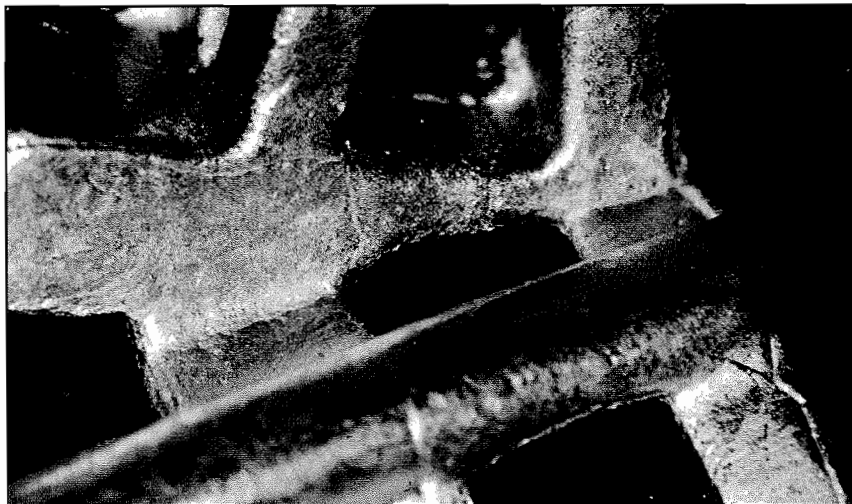
Fig. 3: Shrinkage in Pt-Co alloy "marquise" setting at intersection of baguette prongs and galleries
