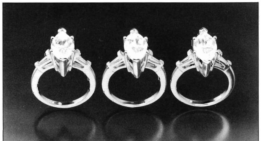
Fig. 2: (Left to right) Finished marquise ring mountings in Pt-Co, Pt-Ru, and Pt-Ir alloys.
