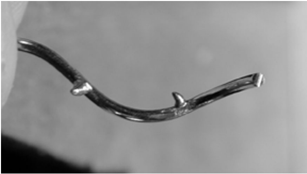
Figure 9: Wire was shaped to create the “stem” of the rose. Thorns are added by soldering (1700 C) the same 16ga. wire to the stem. Clip off the wire, and shape to resemble thorns.
