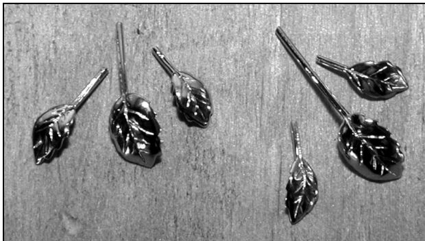
Figure 5: Here the leaves are showing the “veining” an actual leaf contains. This was accomplished with a hart burr to shape and carve. A groove was added in the connector wires themselves. Each element was high polished before assembly, Advantedge polishing pins were used.
