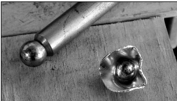
Figure 7: Placing 18ga. sheet into a pitch pot, and using a steel dapping tool, the rose “cup” is formed to fit the cast glass rose, annealing often as I went.
