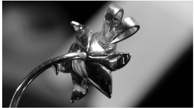
Figure 10: The rose cup detail is visible here. It has been soldered to the stem (1500 C) and a “split” bail has been fabricated and attached (1200C).
