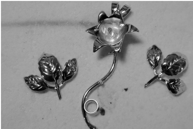
Figure 11: Checking the layout after the bail is attached, insures that bezel placement will be correct. The leaf assemblies as well.
