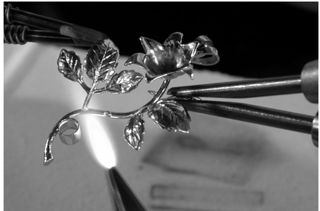
Figure 12: Attaching the bezel and leaf assemblies. (1200 C) Visible is the base of the stem. Welding a scrap piece of Platinum onto the 16ga wire, thickened it enough so it could be shaped to form the base of the stem.
